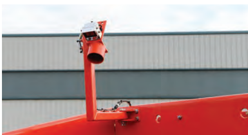
Camera and level sensor to ensure continuous feed
