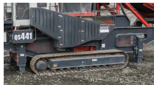
Four jacking legs for increased servicing capabilities
