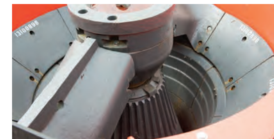
MC chamber with extremely large feed opening
