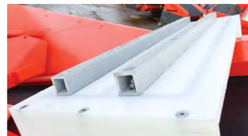
Bridge coil metal detector for controlled detection
