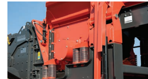
Double deck vibrating pre screen
