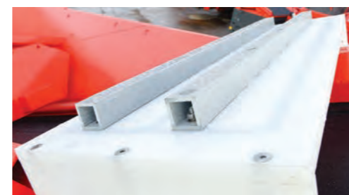
Bridge coil metal detector for controlled detection
