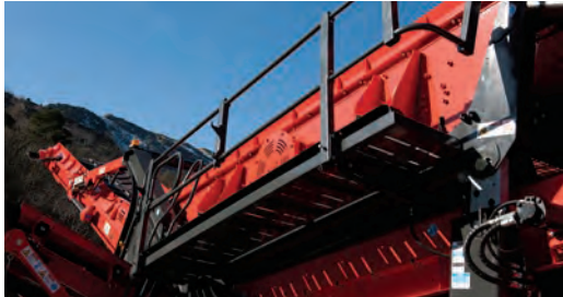
Hydraulically folding maintenance platforms
