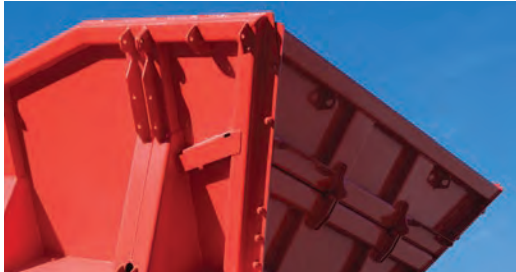
Split rear hopper door for direct feeding
