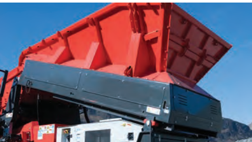
One piece hopper for quick and easy set-up
