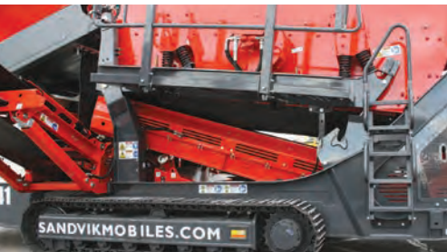
Screen box jack up facility allows easy access
