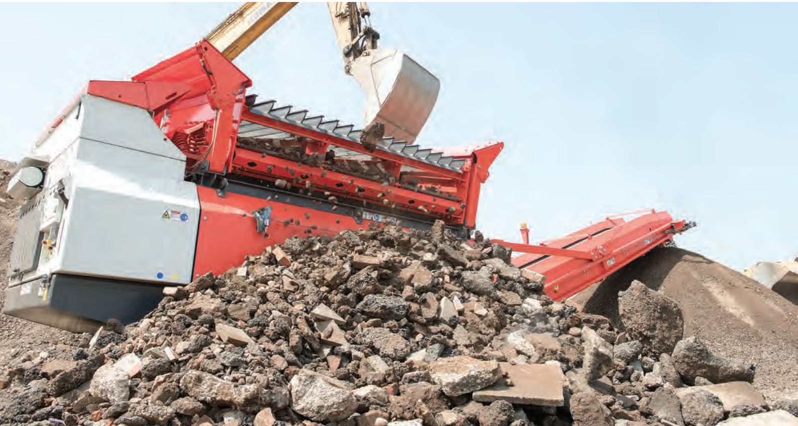
Proven, high performing heavy duty double deck vibrating grid.
