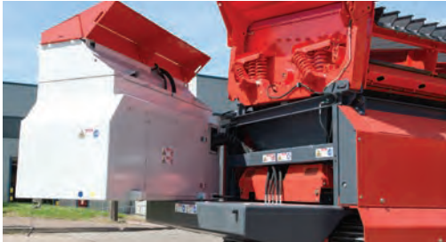
Hydraulically opening powerpack for ease of maintenance
