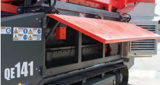
Hydraulically folding doors for easy access
