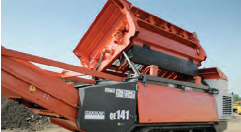
Tipping function activated by radio remote control
