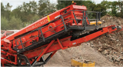
Hydraulically folding walkways for ease of maintenance
