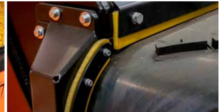
Sealing in the hopper prevents material from leaking to the inside of the machine
