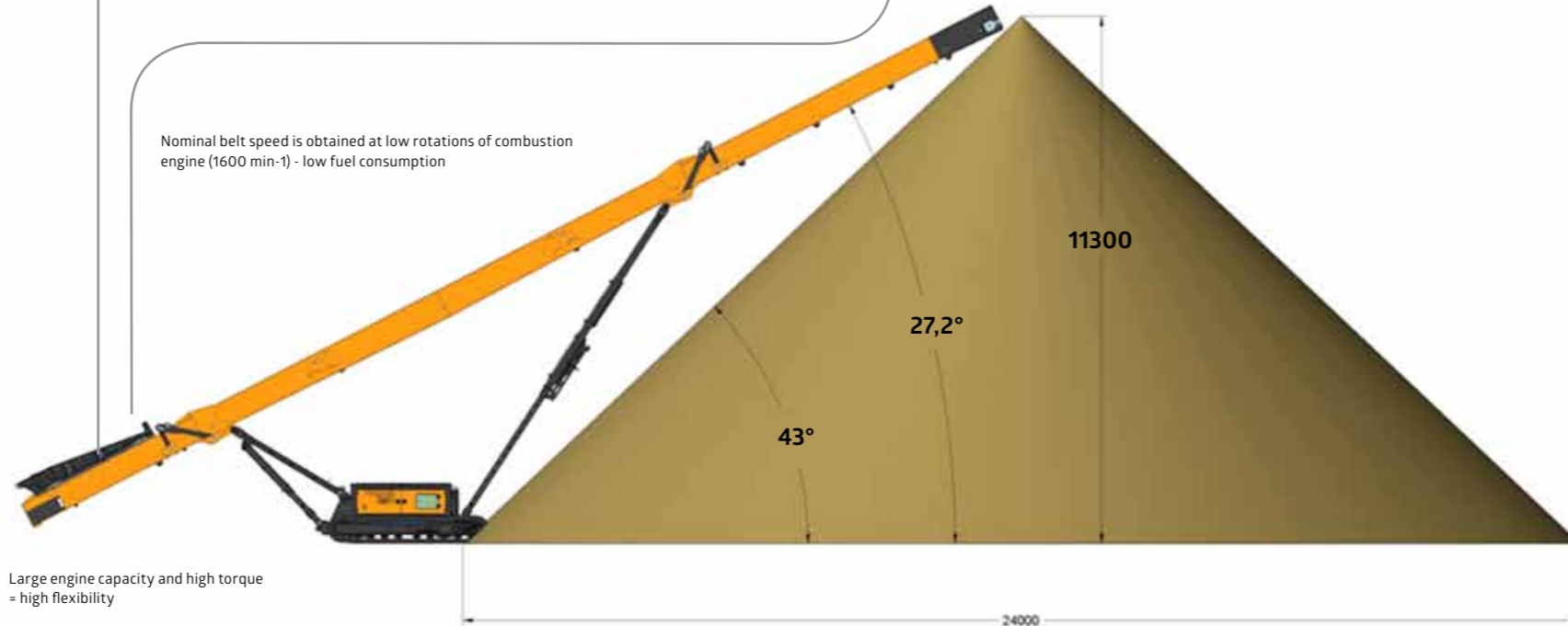
Theoretical maximum volume of 1700 m 3 cone. When storing gravel with density 1600 tons / m 3 , the pile contains 2725 tons of material. The weight of the raw material on the pile depends on material
