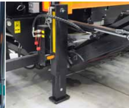
Hydraulic support legs improve machine stability on uneven ground
