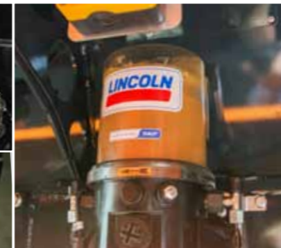
Central lubrication system ensures good greasing of most important parts of the machine
