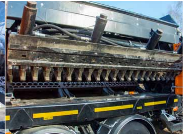
Easily accessible shedding chamber for cleaning or changing counter knives.
