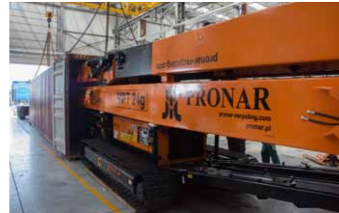
The compact design allows transport in a 40 feet HQ container
