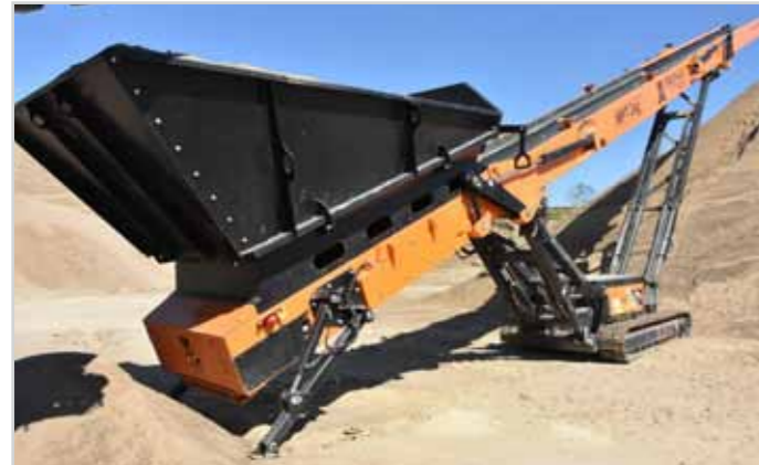
Support legs of the stockpiler improve safety and stability of the machine. Available options: hydraulic (on the photo) or mechanical
