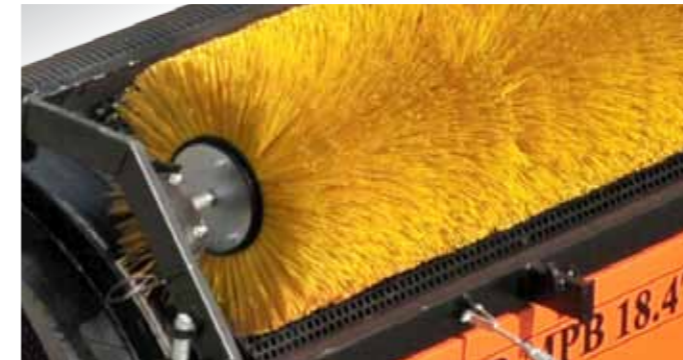
Hydraulically raised and lowered trommel cleaning brush
