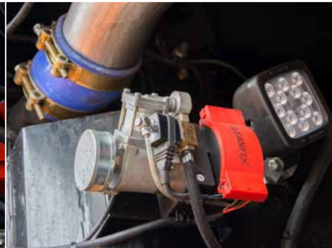
Cleanfix. Facilitates work in difficult conditions - automatic cleaning of oil cooler
