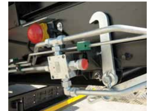
Belt speed adjustment - adjusts the speed to the type of screened material to maximize the performance. It also allows to stack more material of each fraction without the need of re-locating the machine
