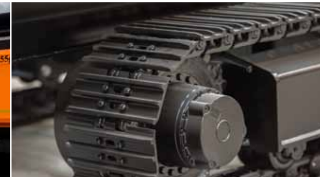
Tracked chassis for moving the machine without any additional towing vehicles
