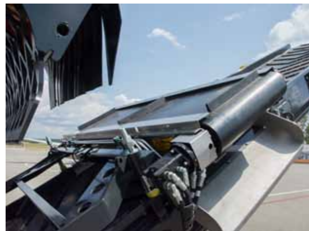
Magnetic separator Use of neodymium magnet ensures effective separation of ferromagnetic material.
