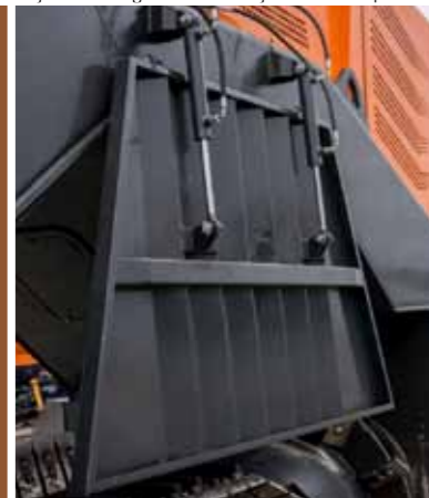
Adjustable tailgate limits the ejection of compost
