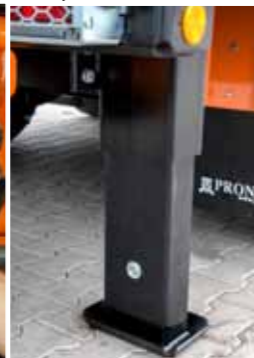
Hydraulic support legs ensures stability of machine
