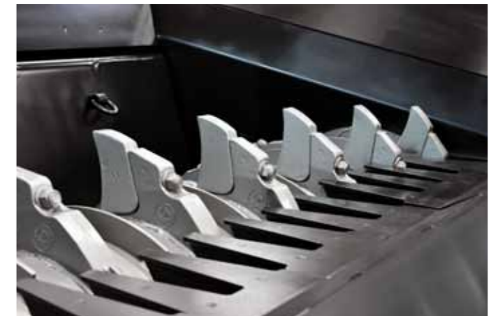
The standard shaft has 42 knife attachment sockets. Assembly and replacement are possible using generally available tools, and exchange is fast.
