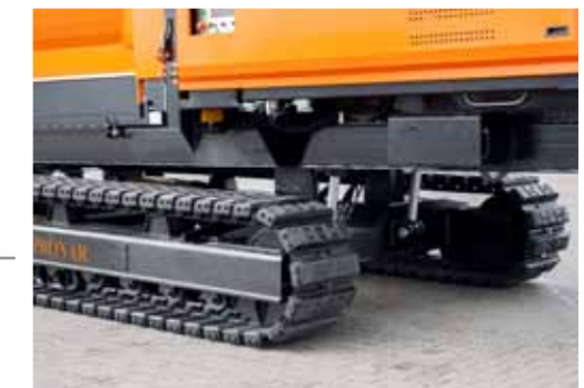
Hydraulic system for adjusting chassis position in MPB 20.55gh. The mechanism allows leveling machine on longitudinal slopes and increases the clearance for easier moving on uneven terrain
