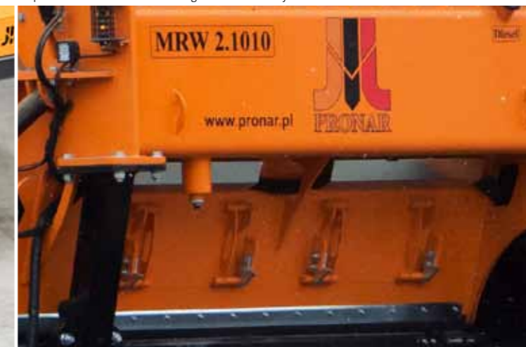
Inspection windows of the working chamber for easy cleanout and maintenance
