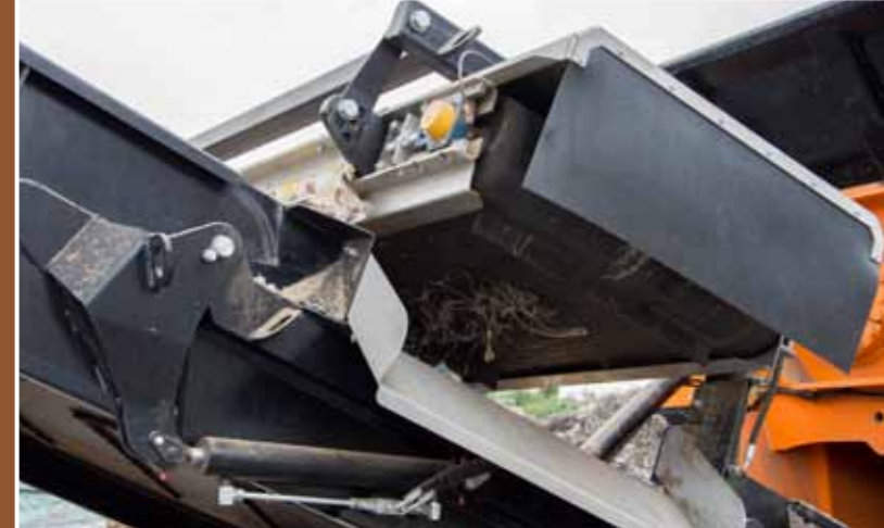
Magnetic separator for extraction of ferromagnetic materials.
