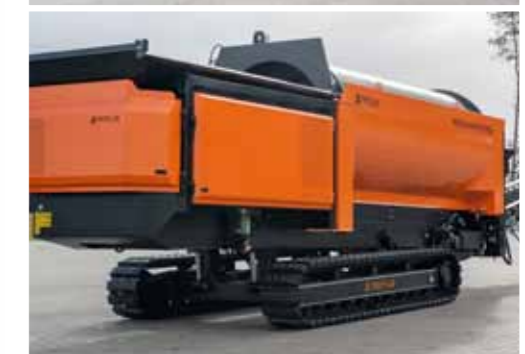
Hydraulic system for adjusting chassis position in MPB 20.55gh. The mechanism allows leveling machine on longitudinal slopes and increases the clearance for easier moving on uneven terrain
