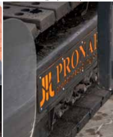
Track drive allows convenient maneuvering of the machine and moving at speeds of up to 4km/h
