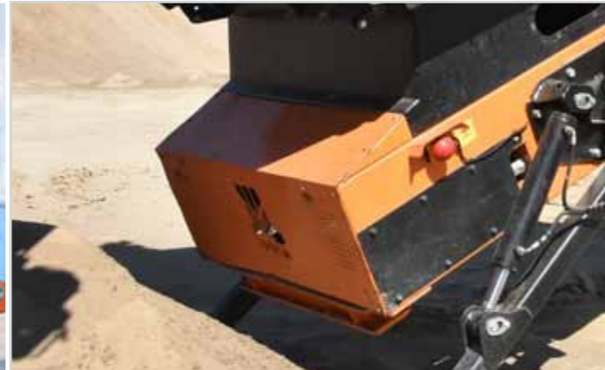
Bumper at the back of the stockpiler protects the shields against damage when leaning construction on the ground (when we do not use the supporting legs)
